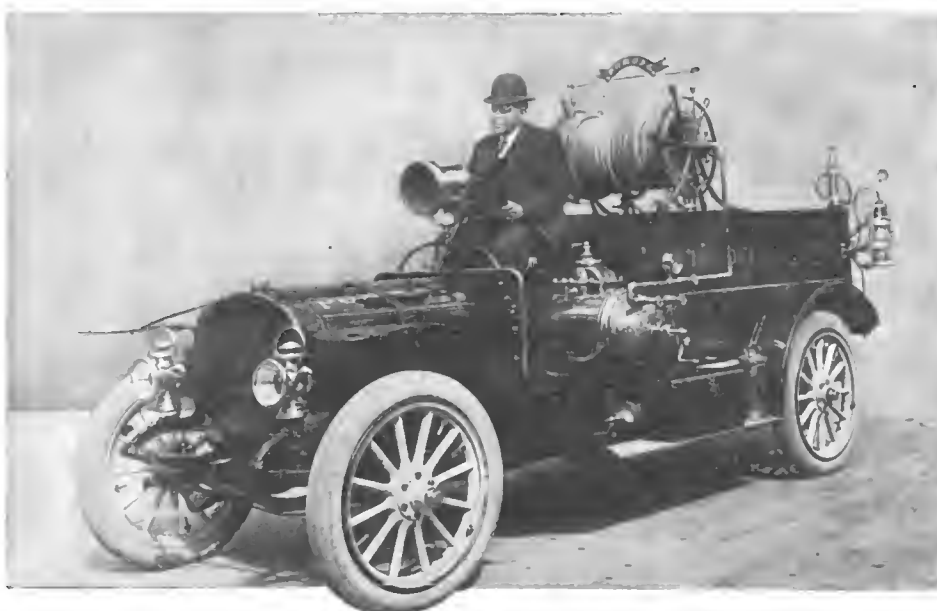
Rambler Chassis with Home-built Body in Service of Pomona, Cal., Fire Department
